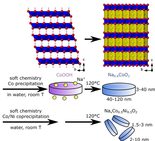
**Figure 1.** Crystal structures of cobalt oxyhydroxide  $\text{CoOOH}$  and three-layer  $\text{Na}_x\text{CoO}_2$  cobaltite (P3 structure). Sodium: yellow, cobalt: blue, oxygen: red, hydrogen: white. The coordination of alkali ions in the P3  $\text{Na}_x\text{CoO}_2$  structure is trigonal prismatic.<sup>3</sup> Schematics of the soft chemistry pathway employed in the present work toward nanoplatelets and nanoflakes of cobaltite and Ni-substituted cobaltite, respectively.
