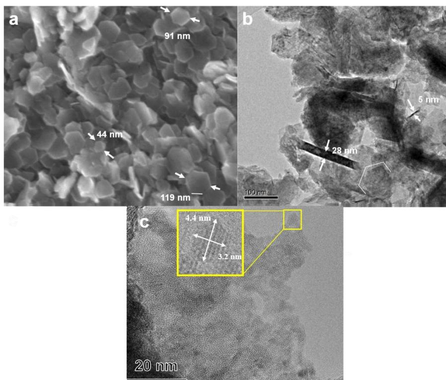
**Figure 3.** Electron micrographs of the  $\text{Na}_{0.6}\text{CoO}_2$  sample: (a) SEM and (b) TEM low magnification image evidencing two different orientations of the nano-platelets in the sample: the basal face and the edge. (c) TEM micrograph of a  $\text{Na}_{0.6}\text{Co}_{0.5}\text{Ni}_{0.5}\text{O}_2$  sample showing in the inset a high resolution magnification of an individual nanoflake.
