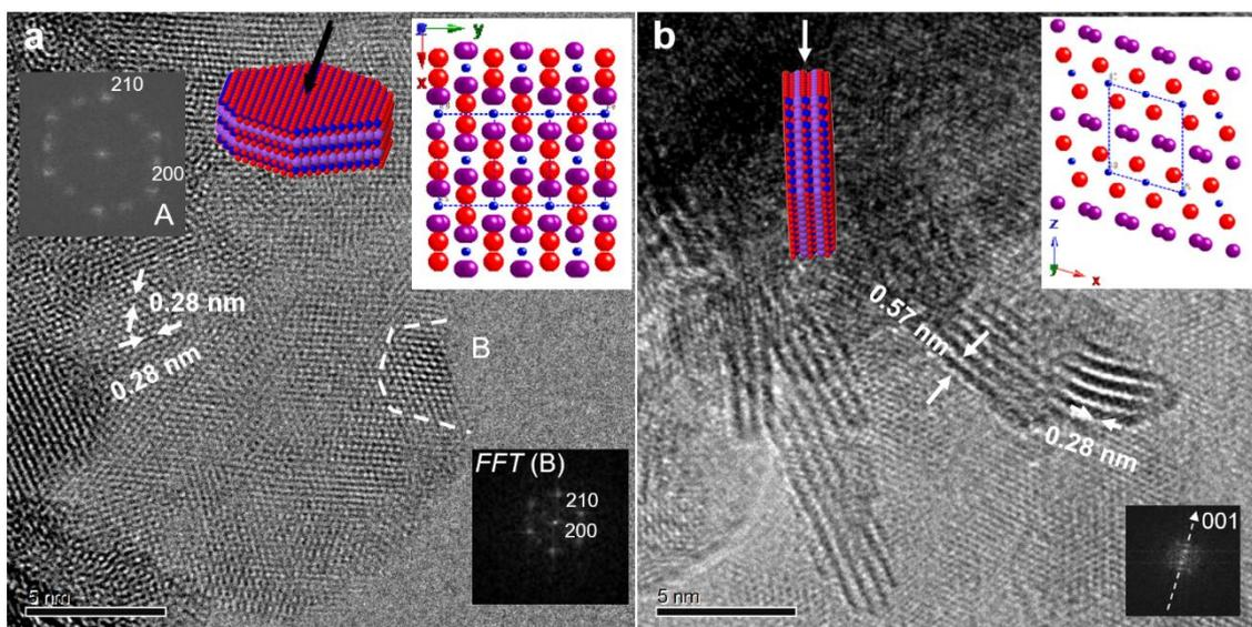
**Figure 4.** HRTEM images of a sample  $\text{Na}_{0.6}\text{Ni}_{0.3}\text{Co}_{0.7}\text{O}_2$ : small nanoflakes orientated along two directions. (a) The [001] projection (zone axis). Notice that due to insufficient thickness, nanoflakes boundaries cannot be observed. (b) The [100] projection (zone axis) of the lamellar  $\text{Na}_x\text{CoO}_2$  system.
