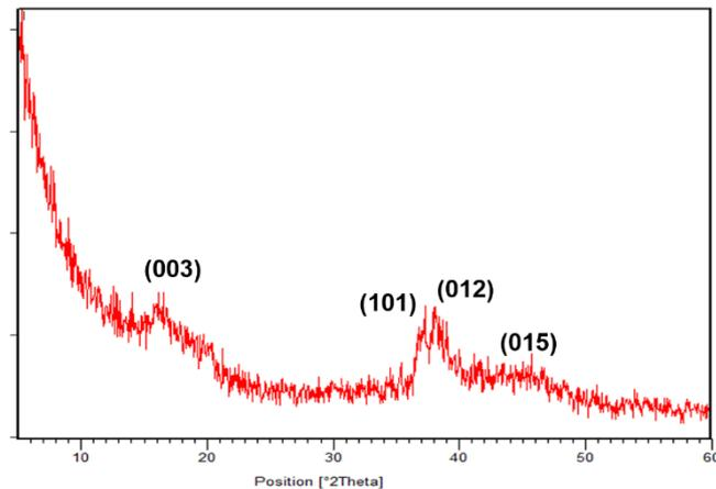
**Figure SI.1.**  $\text{Na}_x\text{Co}_{0.5}\text{Ni}_{0.5}\text{O}_2$  XRD pattern indexed as  $\text{Na}_{0.6}\text{CoO}_2$  (C2/m). Note that the bad signal-to-noise ratio originates from the fluorescence of cobalt and the emission wavelength of the copper anode of the XRD apparatus.
