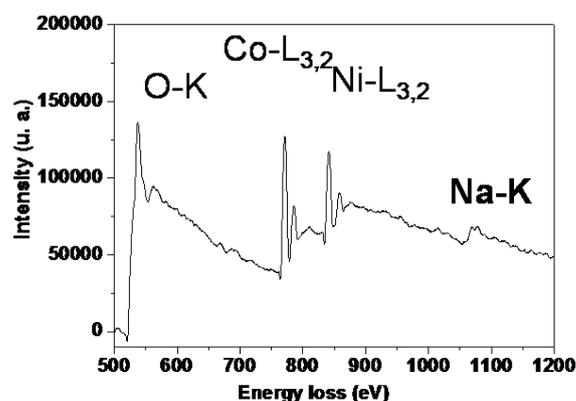
**Figure 7.** Representative EELS spectra for  $\text{Na}_{0.6}\text{Ni}_{0.5}\text{Co}_{0.5}\text{O}_2$ , showing the O-K, Co-L<sub>3,2</sub>, Ni-L<sub>3,2</sub> and Na-K edges.
