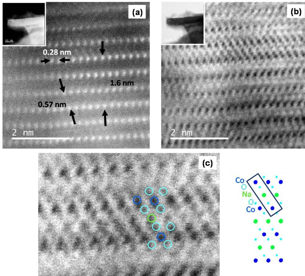
**Figure 5.** Characteristic atomically resolved STEM images of a nanoplatelet in a sample  $\text{Na}_{0.6}\text{Ni}_{0.3}\text{Co}_{0.7}\text{O}_2$  with (a) HAADF and (b) ABF detections. (c) Magnified STEM-ABF image with a schematic representation of the atom distribution along this [100] projection.
