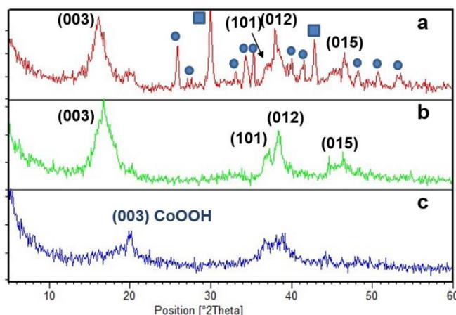
**Figure 2.** XRD patterns of Na<sub>0.6</sub>CoO<sub>2</sub> samples: (a) as-prepared sample, (b) sample after washing with methanol and (c) sample washed before thermal treatment. In (a) and (b), (hkl) indexes correspond to Na<sub>0.6</sub>CoO<sub>2</sub>. Squares correspond to NaBr and circles correspond to Na<sub>2</sub>CO<sub>3</sub>. The indexes in (c) correspond to CoOOH.
