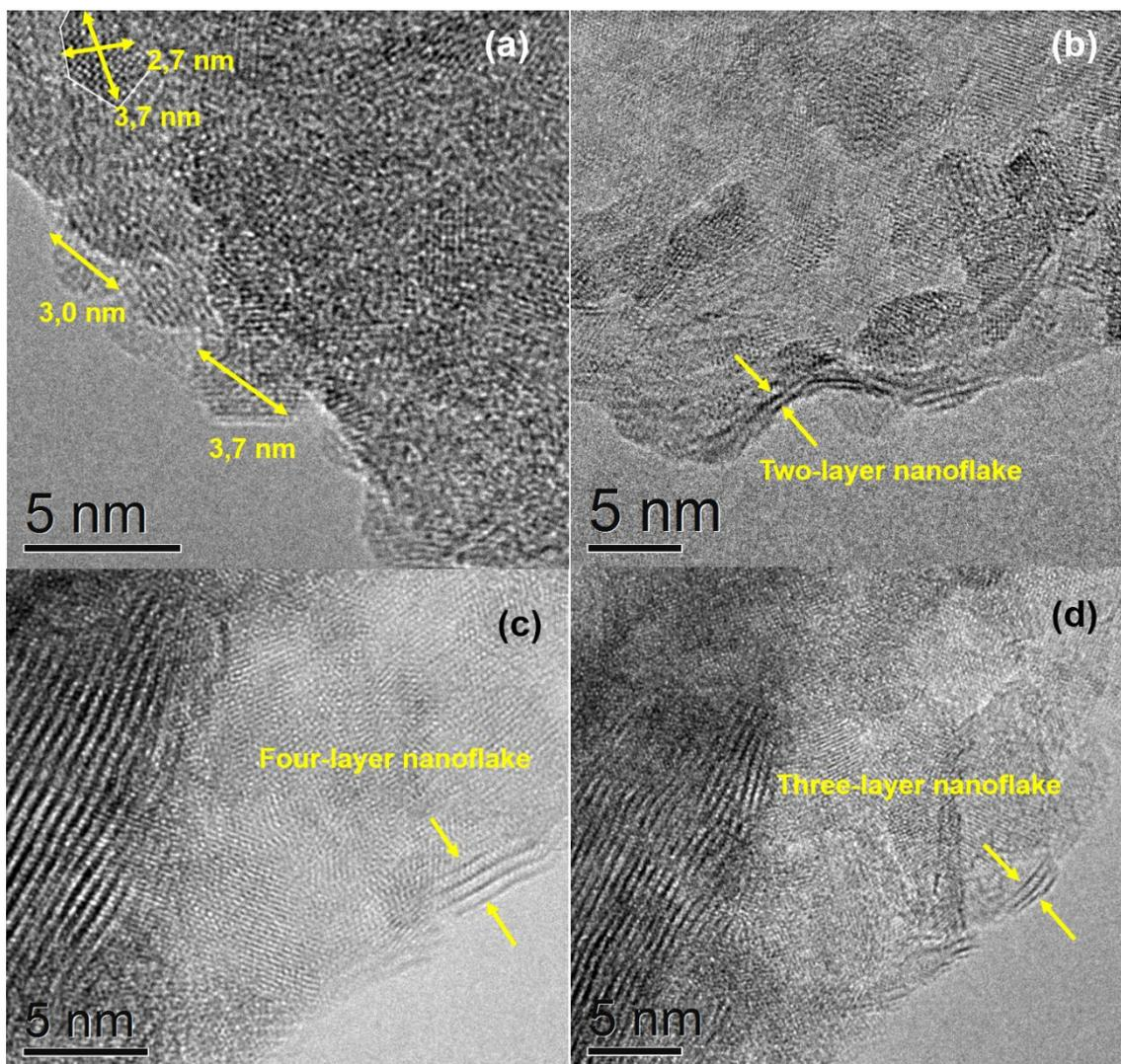
**Figure SI.3.** HRTEM images of a  $\text{Na}_x\text{Ni}_{0.3}\text{Co}_{0.7}\text{O}_2$  sample: small particles orientated along two directions: (a) the [001] projection (zone axis). (b-d) the [100] projection (zone axis) of the lamellar  $\text{Na}_x\text{CoO}_2$  system.
