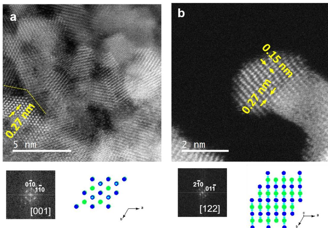
**Figure SI.4.** (a) HAADF image of a group of nanoflakes representative of a sample  $\text{Na}_{0.6}\text{Ni}_{0.5}\text{Co}_{0.5}\text{O}_2$  as well as the FFT of the highlighted area and its structural model. (b) HAADF image of an isolated nanoflake oriented along the [122] direction with its FFT and the structural model along that direction.
