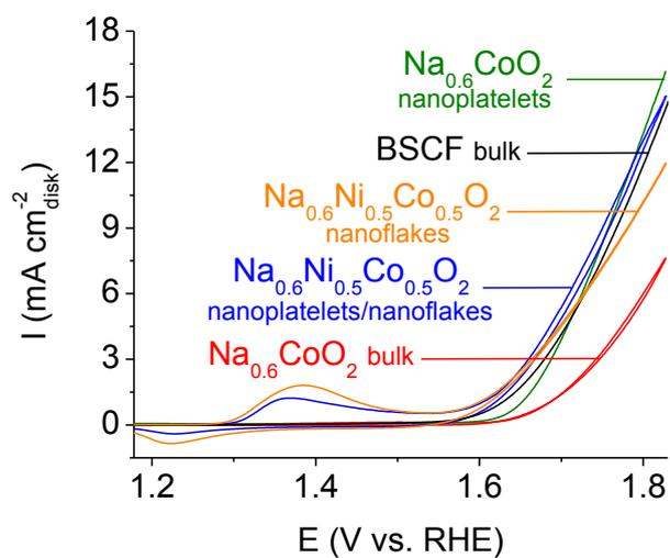
**Figure SI.6.** First linear sweep voltammetry scans ( $20 \text{ mV} \cdot \text{s}^{-1}$ ) of bulk BSCF (black), bulk  $\text{Na}_{0.6}\text{CoO}_2$  (red),  $\text{Na}_{0.6}\text{CoO}_2$  nanoplatelets (green),  $\text{NaNi}_{0.5}\text{Co}_{0.5}\text{O}_2$  mix of nanoplatelets and nanoflakes (blue),  $\text{NaNi}_{0.5}\text{Co}_{0.5}\text{O}_2$  nanoflakes (orange).
