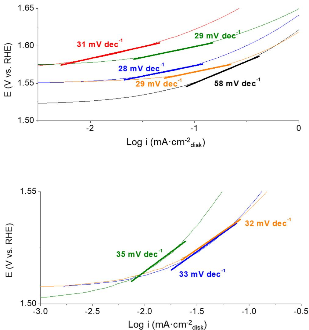
**Figure SI.8.** Tafel plots at the 5<sup>th</sup> linear sweep voltammetry scan (top,  $20 \text{ mV}\cdot\text{s}^{-1}$ ) and after 5h chronopotentiometry (bottom,  $5 \text{ mA}\cdot\text{cm}^{-2}$ ) of bulk  $\text{Na}_{0.6}\text{CoO}_2$  (red),  $\text{Na}_{0.6}\text{CoO}_2$  nanoplatelets (green),  $\text{NaNi}_{0.5}\text{Co}_{0.5}\text{O}_2$  mix of nanoplatelets and nanoflakes (blue),  $\text{NaNi}_{0.5}\text{Co}_{0.5}\text{O}_2$  nanoflakes (orange).
