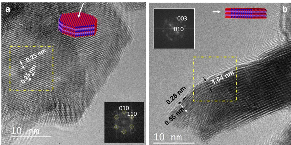
**Figure SI.2.** HRTEM images of a  $\text{Na}_{0.6}\text{CoO}_2$  sample. (a) Nanoplalets oriented along [001] and corresponding FFT of the highlighted area. (b) Nanoplalete oriented along [100] and corresponding FFT of the highlighted area.
