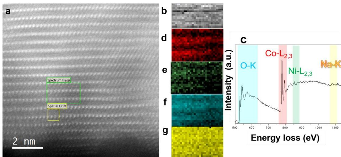
**Figure 6.** (a) HAADF detail of a  $\text{Na}_{0.6}\text{Ni}_{0.3}\text{Co}_{0.7}\text{O}_2$  nanoplatelets. (b) Simultaneously acquired image. (c) Sum spectrum. (d-g) Chemical maps obtained in the green square in (a) from the Co-L<sub>2,3</sub>, Ni-L<sub>2,3</sub>, O-K and Na-K edges, respectively.
