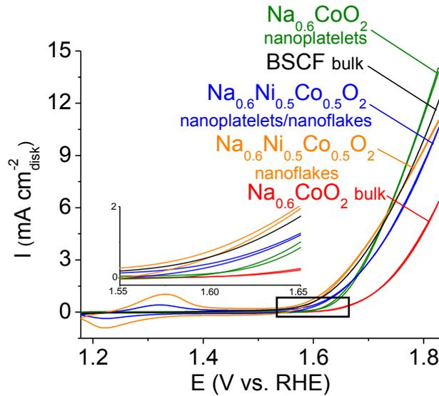
**Figure 8.** 5<sup>th</sup> linear sweep voltammetry scans ( $20 \text{ mV}\cdot\text{s}^{-1}$ ) of bulk BSCF (black), bulk  $\text{Na}_{0.6}\text{CoO}_2$  (red),  $\text{Na}_{0.6}\text{CoO}_2$  nanoplatelets (green),  $\text{Na}_{0.6}\text{Ni}_{0.5}\text{Co}_{0.5}\text{O}_2$  mix of nanoplatelets and nanoflakes (blue),  $\text{Na}_{0.6}\text{Ni}_{0.5}\text{Co}_{0.5}\text{O}_2$  nanoflakes (orange). The inset shows a zoom in of the onset potential area.
