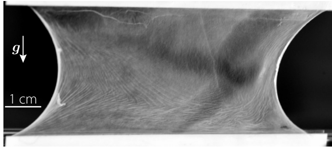
Figure S18: Thick PAN membrane wicked with a large amount of water. Unlike the case presented in Figure S17, gravity now is oriented in the same direction as the compression axis of the membrane. This results in a wrinkling pattern where again, the preferred directions follow the circular arcs of the free edges. It should be noted that the inhomogeneities in the membrane's color density correspond differences in thickness, but they do not affect the wrinkling pattern significantly.
