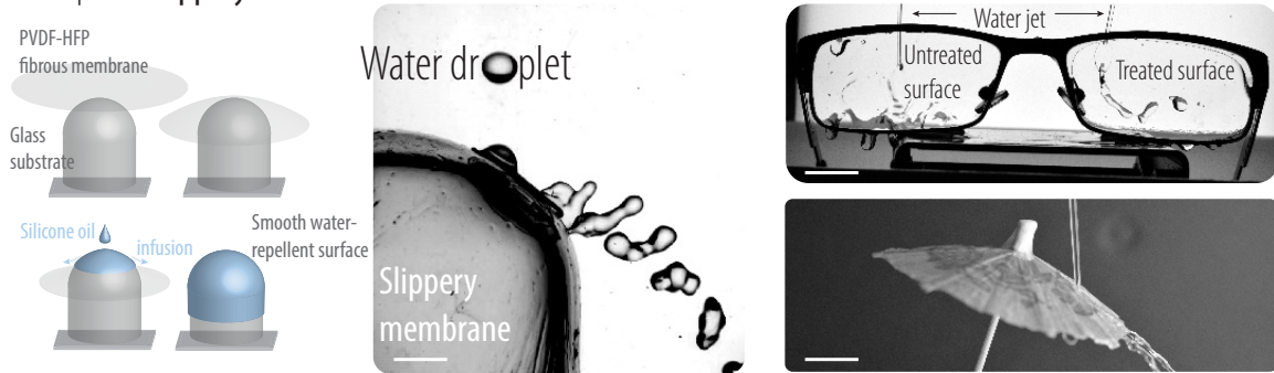
Figure 4: Stretchable electronics, on-demand contractibility and adaptable slippery surfaces. A. A thin gold strip (100 nm thick) is apposed on the wicked membrane (here : PVDF-HFP membrane wicked by \nu 100 silicone oil). Capillary adhesion guarantees the gold strip to remain secured to the membrane. Electricity runs through the gold strip even when membrane reserves are spontaneously generated upon compression of the membrane. Electric resistance versus membrane extension X is presented in the graph and due to local short circuits, this resistance drops as the membrane is contracted. Indeed, as shown on the right photograph (scale bar: 7 mm), a gold strip wrinkles and folds when the membrane is compressed. The sequence shows the illumination of a 1.5V LED through a basic electric circuit throughout an 8-fold extension of the supporting wicked membrane. Scale bar: 3cm. B. Capillary contraction upon wetting. The dry membrane is here attached to two mobile supports (rafts freely gliding on a water bath, first photograph). When ethanol (dyed blue for visualization) is sprayed on the membrane, membrane reserves are immediately generated through the capillary action; the two mobile rafts are pulled towards one and other. Scale bar: 3cm. C. A PVDF-HFP fibrous membrane is apposed to a non-flat surface and is wicked by silicone oil. Capillary adhesion secures the wicked membrane onto the surface and the spontaneous generation of surface reserves allow for a macroscopically smooth surface even on a warped surface (folds are confined in the liquid film). The wicked membrane then acts as a slippery surface treatment with water repellent properties. The chrono-photography (10 ms intervals, scale bar: 7mm) shows a water droplet bouncing off such a treated spherical glass surface. The wicked membrane can adapt to any object such as glasses (scale bar: 1.5 cm, water droplets stick to the untreated surface but roll off the treated glass) or cocktail umbrellas (scale bar: 2cm, the water repelling property is conserved after consecutive opening/closing of this toy umbrella).
