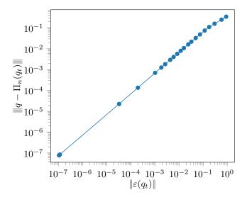
FIGURE 4. Fourth test case: Projection error as a function of the error polynomial amplitude  $\|\varepsilon(q_t)\|$ , which measures the distance of the Lukàcs quaternion  $q_t$  to the desired lower and upper bounds. Here the experimental convergence rate  $\approx 1$  (that is the slope of the line) is much better than what is predicted by Theorem 4.1 which is a slope  $\approx \frac{1}{2^{11}}$  for n=5.
