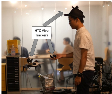
Figure 4: HTC Vive Motion Capture Setup
