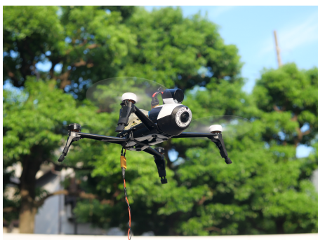
Figure 1: Flying tethered drone with prolonged flight time
