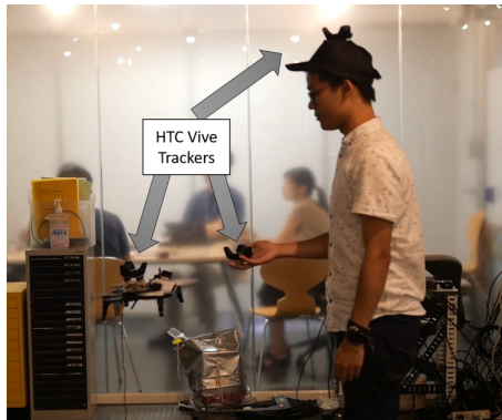
Figure 4: HTC Vive Motion Capture Setup
