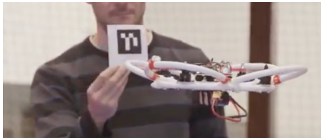
Figure 9: Drone automatically orienting itself towards a marker.
