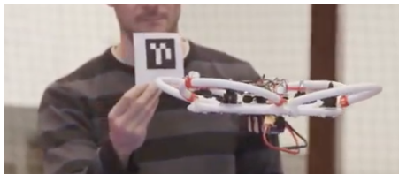
Figure 9: Drone automatically orienting itself towards a marker.
