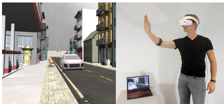
Figure 2: Person interacting with automated vehicles in a VR Simulation - interacting with an automated vehicle to indicate it should give way.
