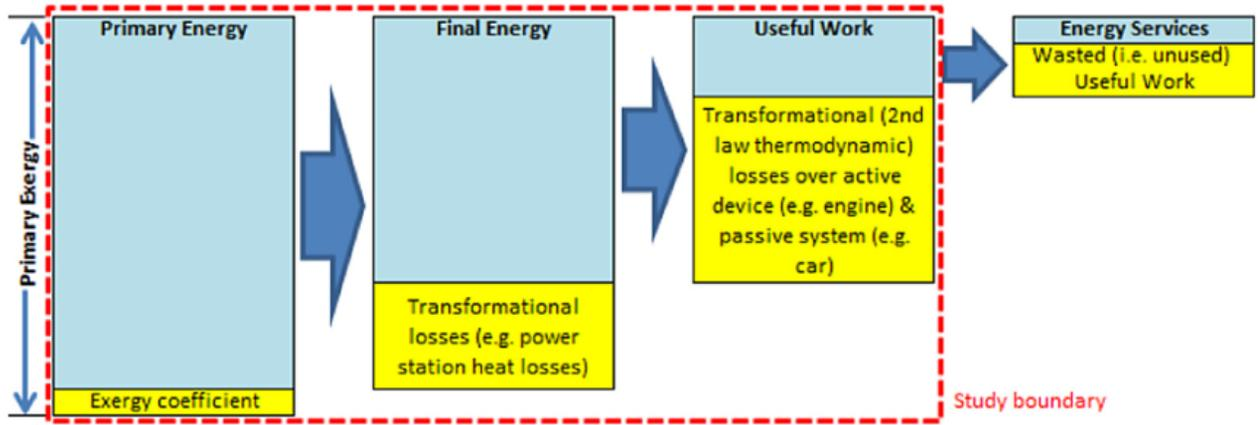
Figure 1: Energy Conversion Chain as considered in this article [Brockway et al., 2015]
