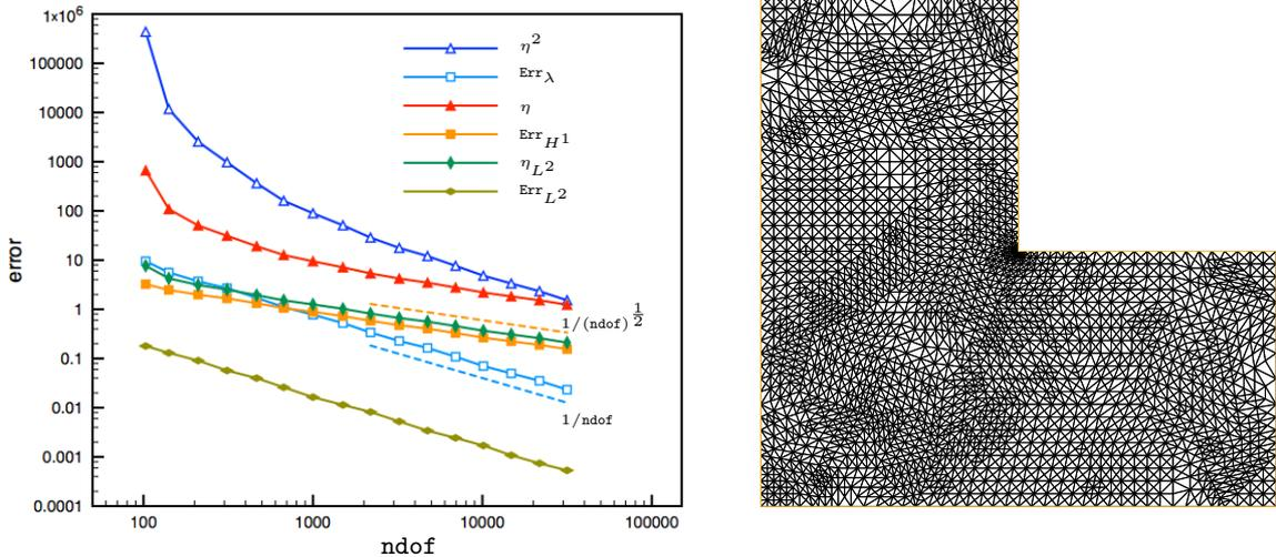
Figure 3: Convergence of various measures of the error and their upper bounds for finite elements on the L-shaped domain with  $m = 3$ ,  $M = 5$  using an adaptive refinement strategy (left). The mesh at the 10th iteration (right).
