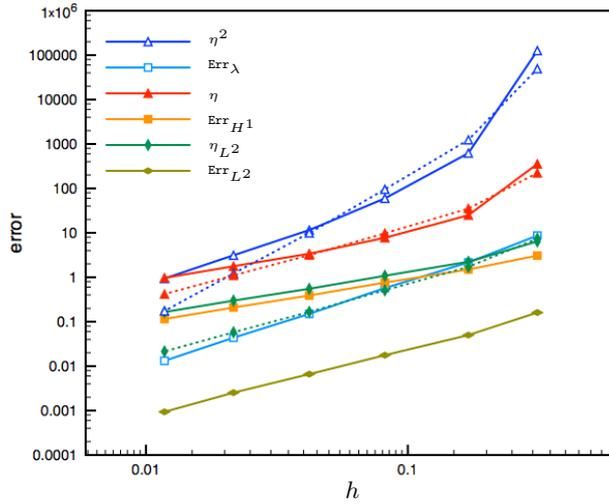
Figure 2: Convergence of various measures of the error and their upper bounds for finite elements and the unit square with  $m = 2, M = 3$  (top) and for the L-shaped domain with  $m = 3, M = 5$  (bottom). The dotted lines provide the estimators using Case II with  $\delta = \frac{2}{3}$  and the empirical choice  $C_S = C_I = 1$ .
