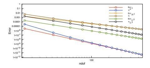
Figure 3: Convergence of the errors and their upper bounds for a 1D Schrödinger operator with periodic boundary conditions with m = 2, M = 3.
