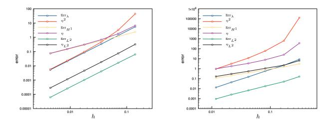
Figure 2: Convergence of various measures of the error and their upper bounds for finite elements and the unit square with m = 2, M = 3 (left) and for the L-shaped domain with m = 3, M = 5 (right).
