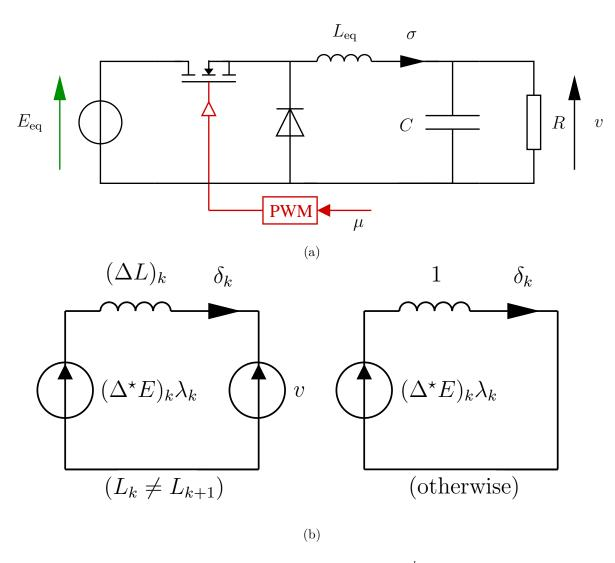
Figure 9: Circuit theory interpretation of (a)  $\Sigma_v$  and (b)  $\Sigma_\delta^k$  in the two cases.
