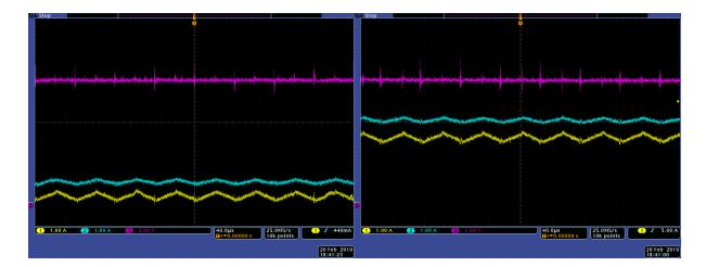
Figure 21: Oscilloscope screen-shots of steady state for  $R=12\Omega$  (left),  $R=1.8\Omega$  (right) ( $i_1$  in yellow,  $i_2$  in cyan, v in magenta).
