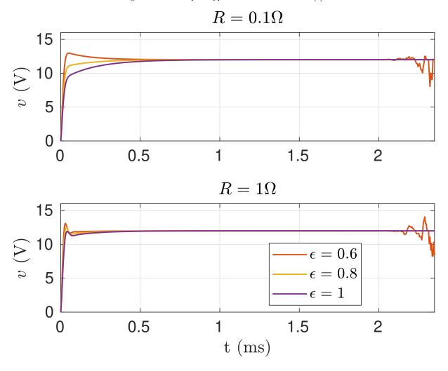
Figure 6: Impact of load value and gain of the outer loop on step response of closed-loop system with two loops controller.
