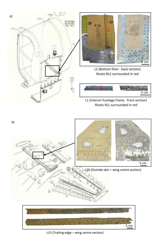
Figure 1. Photographs of collected parts (front and back side) from Breguet 765 airplane with localization on original plans (Breguet n.d.); a) Plate L2 (2 mm thick) with RL2 rivets (5 mm diameter) and profile L1 with RL1 rivets (4 mm diameter), b) Plate L20 (3 mm thick) and profile L15 (4 mm thick); c) Plate L8 (1.6 mm thick) and bracket L9 (5 mm thick).
