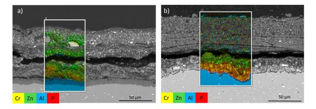
Figure 1. Coating detected in L9 (back side) and L15 (front side) with SEM: backscattering image and EDS maps. Only Zn, P, Cr and Al are shown. In blue: Al-alloy, green: zinc, yellow: chrome and red: phosphorus.
