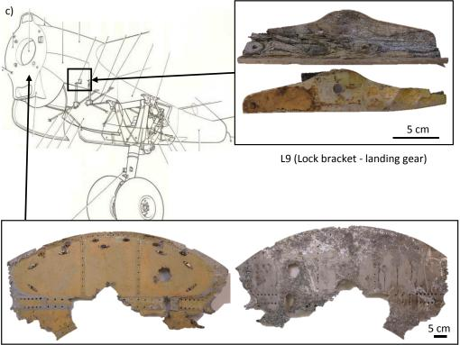
L8 (Flame shield - engine nacelle)
