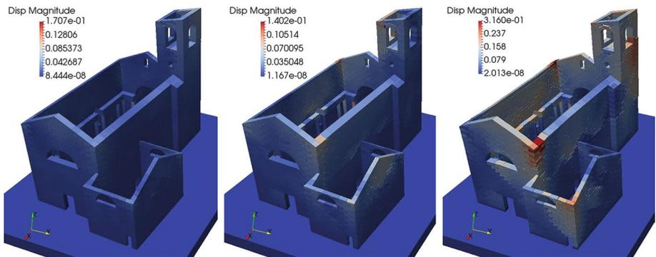
**Fig. 20** Damages of the Church of San Francesco in Sarnano (MC) under the earthquakes of 24th August 2016 (a), 26th October 2016 (b), and 30th October 2016 (c)
