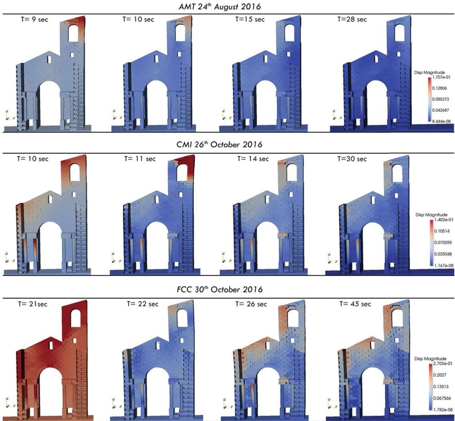
Fig. 21 Shear mechanisms in the triumphal arch of San Francesco in Sarnano (MC)
