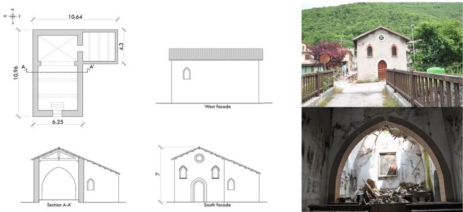
Fig. 5 Geometric configuration of Sant'Antonio's church, Ussita
