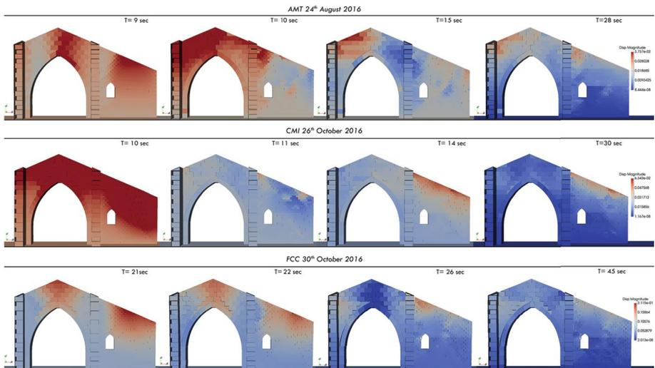
Fig. 30 Shear mechanisms of the triumphal arch of Sant'Antonio in Ussita (MC)
