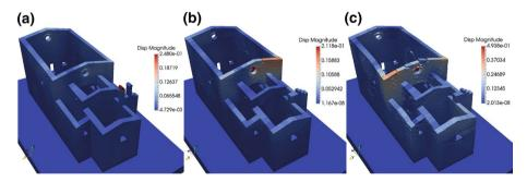
Fig. 32 Damages of the sanctuary of Madonna of Valcora in Fiuminata (MC)under the earthquakes of 24th August 2016 (a), 26th October 2016 (b), and 30th October 2016 (c)
