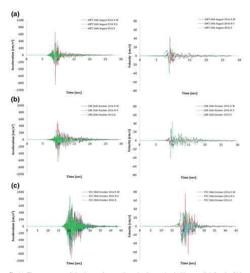
**Fig. 14** The components of the three main ground accelerations and velocities recorded for: the 24th August 2016 Earthquake in the station of Amatrice (AMT) (**a**), the 26th October 2016 Earthquake in the station of Campi (CMI) (**b**), and the 30th October 2016 Earthquake in the station of Forca Canapine (FCC) (**c**)
