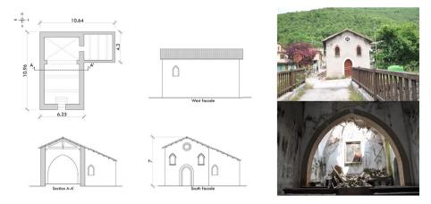
Fig. 5 Geometric configuration of Sant'Antonio's church, Ussita
