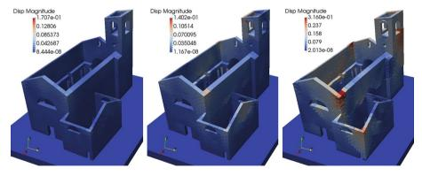
Fig. 20 Damages of the Church of San Francesco in Sarnano (MC) under the earthquakes of 24th August 2016 (a), 26th October 2016 (b), and 30th October 2016 (c)
