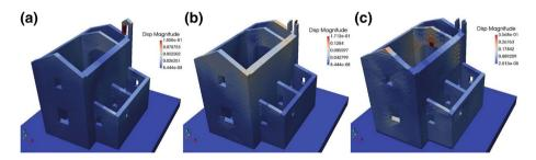
Fig. 24 Damages of the Church of Sant'Anna in Camerino (MC) under the earthquakes of 24th August 2016 (a), 26th October 2016 (b), and 30th October 2016 (c)
