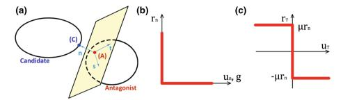
Fig. 12 Relation between candidate and antagonist in 3D space (a), Signorini's impenetrability condition (b), and friction à la Coulomb (c)
