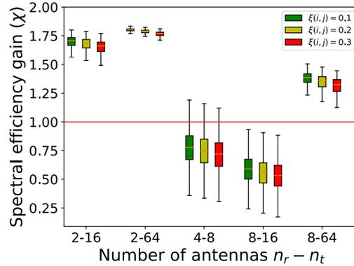
FIGURE 2: Spectral efficiency gain of MU-MIMO over SU-MIMO
