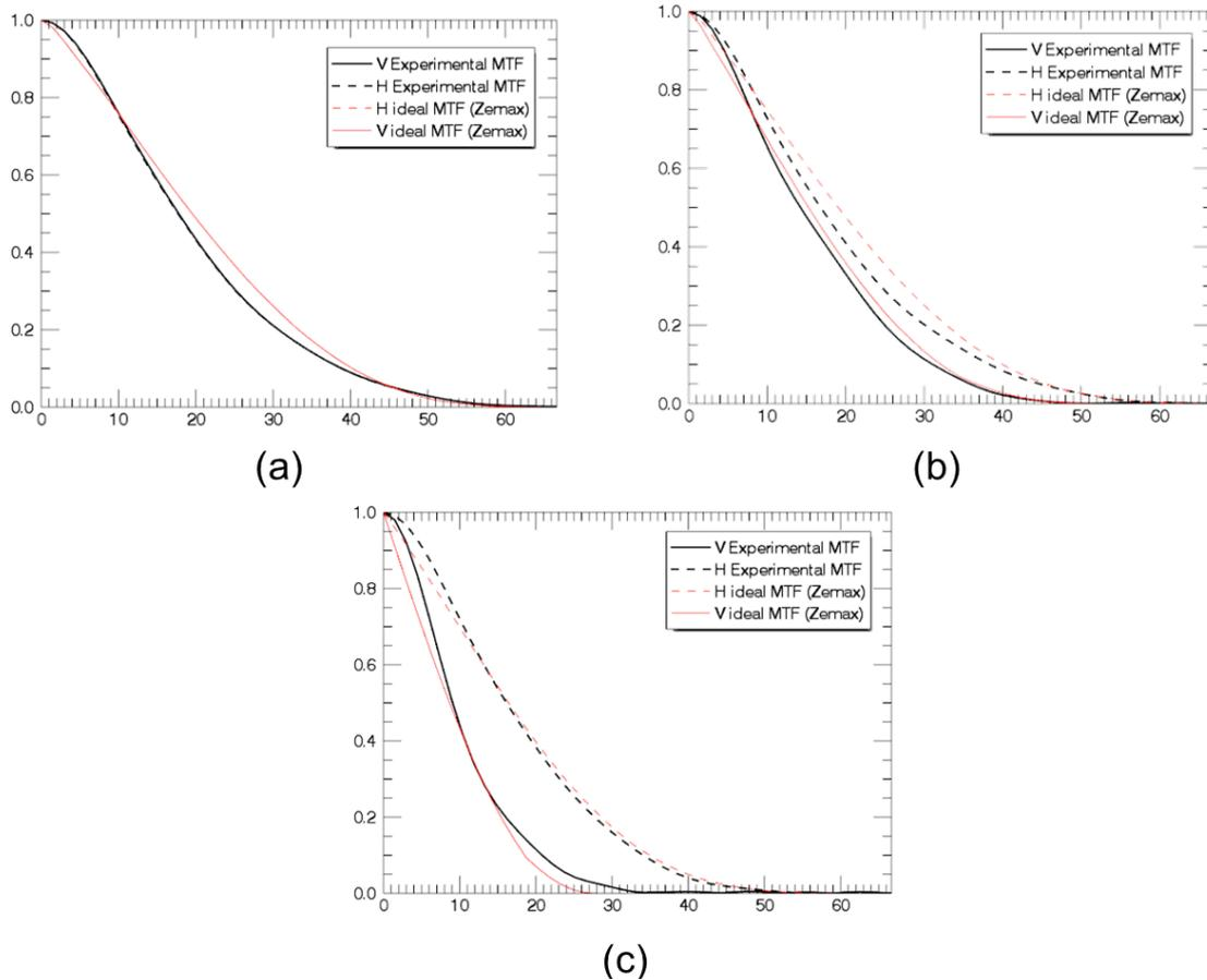
Figure 5 – MTF plots for different field angles ( $\theta$ ) inside the central microlens. Spatial frequencies along the horizontal axis are given in cycles/mm. (a) On axis,  $\theta=0^\circ$ . (b)  $\theta=0.73^\circ$ . (c)  $\theta=1.17^\circ$
