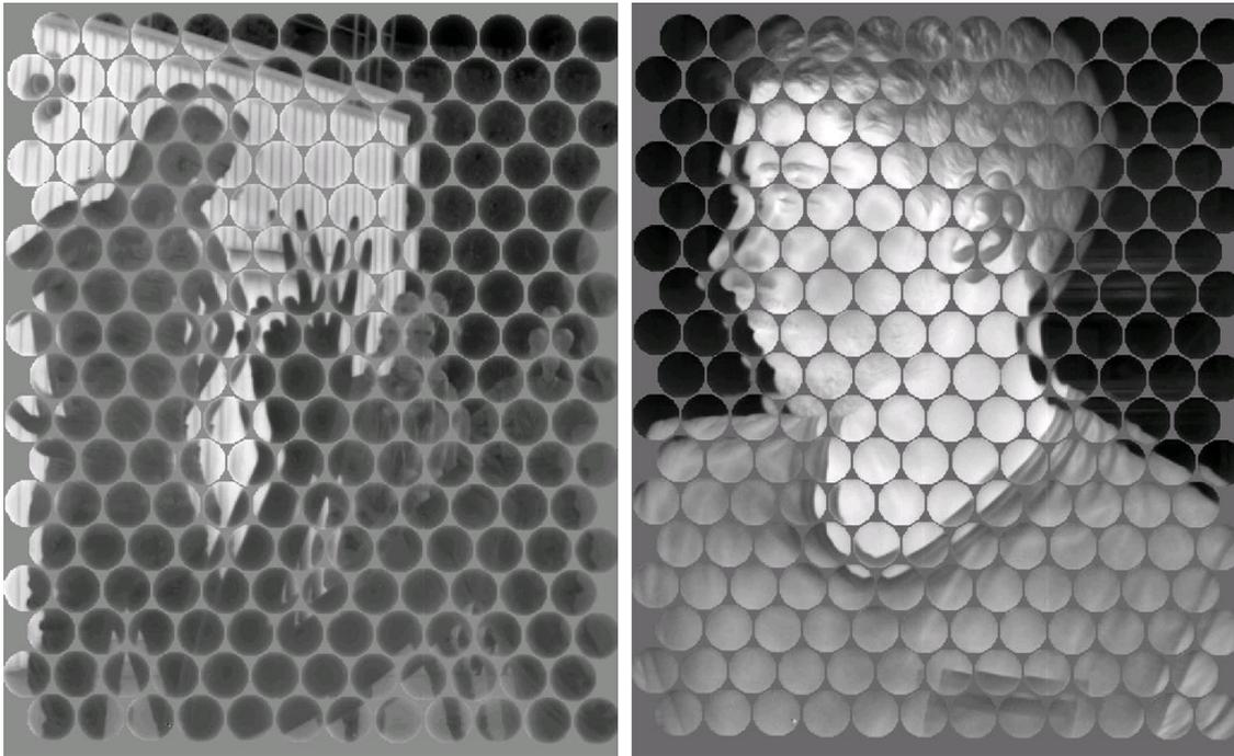
Figure 8 – Images taken with our infrared plenoptic camera
