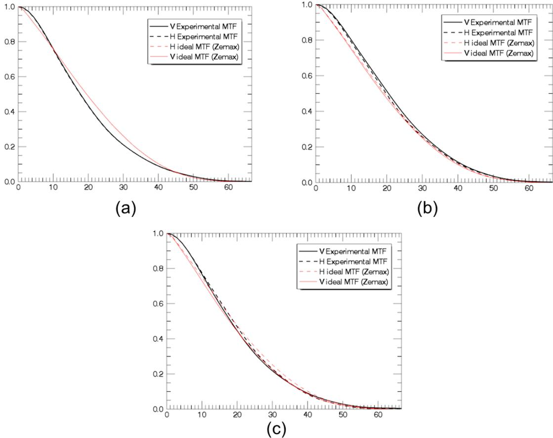
Figure 7 – On axis MTF plots for different microlenses in the array. Spatial frequencies along the horizontal axis are given in cycles/mm. (a) On axis,  $\theta=0^\circ$ . (b)  $\theta=8^\circ$ . (c)  $\theta=11^\circ$
