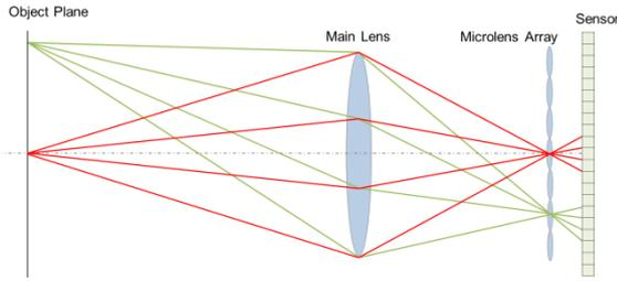
Figure 2 - The plenoptic 1.0 camera: a single object point is seen by several pixels behind a single microlens.
