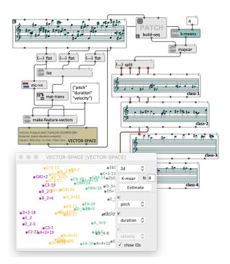
Figure 2. A simple example of clustering applied to a sequence of notes. Feature-vectors are formatted and input to the VECTOR-SPACE object. From there, the *k-means* algorithm clusters the data based on the specified features (*pitch*, *duration*, *velocity*). Vectors are output and split by clusters to generate four separate voices.
