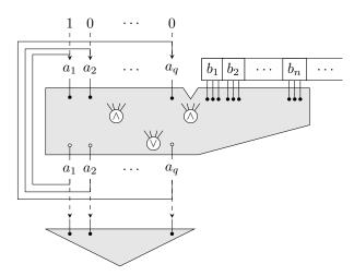
Such a streaming circuit can be interpreted as a deterministic automaton over the alphabet  $\Gamma = \Sigma^n$ : the state space is  $\{0, 1\}^m$  with the initial state  $10^{m-1}$ , and the transition function and the set of accepting states are given by circuits C and A. Consequently, languages recognized by streaming circuits are regular.
