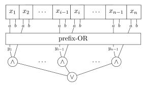
This construction can be nested: for the language of words having at least k occurrences of a, one uses k prefix-OR circuits with n inputs interleaved with k layers of AND gates of fan-in 2, with the last layer of AND gates connected to a single OR gate. The size of the resulting circuit is therefore  $\mathcal{O}(kn)$  and is independent from the size of the input alphabet.
