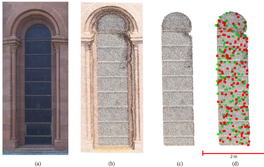
Figure 6. The steps in the keypoint detection and matching: (a) image of an example window opening. Here is shown the exterior side; (b) segmented point cloud of this window; (c) window pane extracted using a RANSAC algorithm; (d) detected SHOT keypoints. Red denotes exterior keypoints and green interior keypoints.
