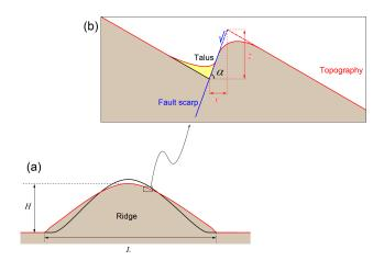
**Figure 2.** Parameters used for calculation of vertical and horizontal displacement across (a) topographic ridge and (b) uphill-facing normal fault scarp. The black lines indicates pre-DSGSD ridge topography and the red lines post-DSGSD topography. H is observed ridge height, L is observed ridge width,  $\alpha$  is fault dip angle, x is horizontal fault displacement, and z is vertical fault displacement.
