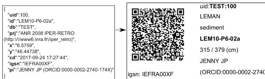
Figure 2: A label sample used for cores of sediments with the associated QR code.
