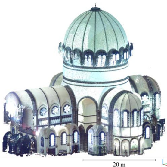
Figure 5. Overview of the colored registered dataset (interior part of the building)
