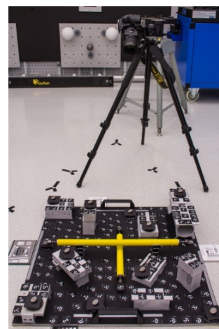
Figure 7: The 3D test object consisted of about 170 coded targets with a largest dimension of 900 mm.
