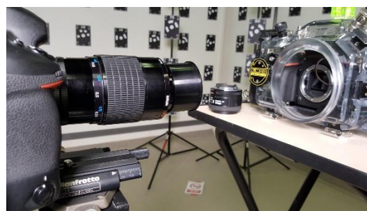
Figure 5. The Nikon D750 DSLR camera with NiMAR NI3D750ZM pressure housing during the measurement of Z_0 in laboratory.
