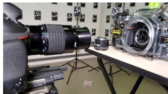
Figure 5. The Nikon D750 DSLR camera with NiMAR NI3D750ZM pressure housing during the measurement of Z_0 in laboratory.
