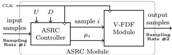
Fig. 1. Simplified high-level architecture of the ASRC module
