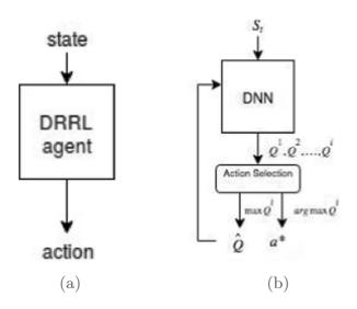
Fig. 1. (a) A top-level view of the DRRL agent algorithm, with the state as input and the preferable action as output. (b) The network gets  $S_t$  as input at time t and outputs all the  $Q^i$ s. Then the action with the maximum  $Q^i$  for this state is returned as output of the algorithm and the maximum  $Q^i$  is used in next network iteration.
