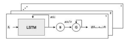
**Fig. 2.** A visualization of the network for one action. The deep network consists of I = |A| parallel RNNs with LSTMs (LSTM layer). A soft-max activator (soft-max layer) follows each one of them in order to normalize weights  $\theta^i$  and the Q-value is updated (Q-value layer). Each RNN outputs a Q-value.
