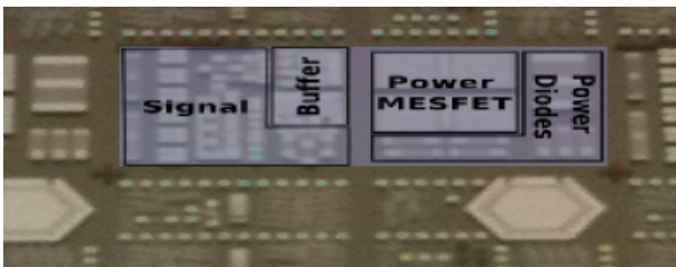
Figure 14 Photography of the elementary field of the SiC integrated power converter (signal-left / control-right)
