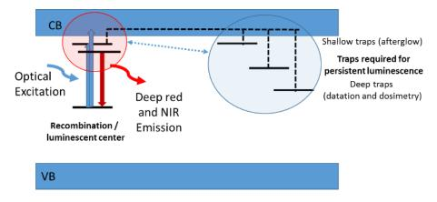
Fig. 2. Schematic of the energy levels and traps involved in the persistent luminescence mechanisms.
