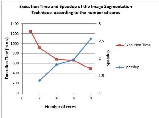
Fig. 14 Execution time and speedup of the parallel Image Segmentation Technique according to the number of cores for a 2048 \times 2048 image
