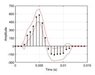
Fig. 5. Finite impulse response model. Each discrete stem represents one coefficient  $h_k$ , upper and lower red dot line constitute the 95% confidence interval. (For interpretation of the references to color in this figure legend, the reader is referred to the web version of this article.)
