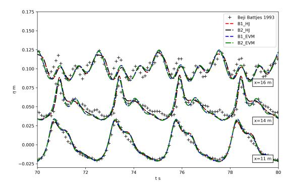
Figure 2 – Time series of the free surface elevation for a test with regular waves (H = 0.054 m, T = 2.5 s). Comparison between experimental measurements and numerical simulations with whispers3D using different combinations of breaking criterion and dissipation method. The curves at each position, x, are offset by 0.05 m for clarity.
