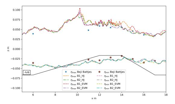
Figure 5 – Comparison of the wave envelops of the experimental data and numerical simulation results for a test with irregular waves ( $H_{m_0} = 0.049 \text{ m}$ ,  $T_p = 2.5 \text{ s}$ ), using different combinations of breaking criterion and dissipation method.
