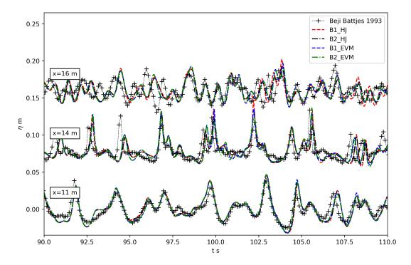
Figure 4 – Time series of the free surface elevation for a test with irregular waves ( $H_{m_0} = 0.049$  m,  $T_p = 2.5$  s). Comparison between experiment and numerical simulations with whispers3D using different combination of breaking criterion and dissipation method. The curves at each position, x, are offset by 0.08 m for clarity.
