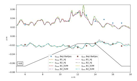
Figure 3 – Comparison of the wave envelops of the experimental data and numerical simulation results for a test with regular waves (H = 0.054 m, T = 2.5 s), using different combinations of breaking criterion and dissipation method.
