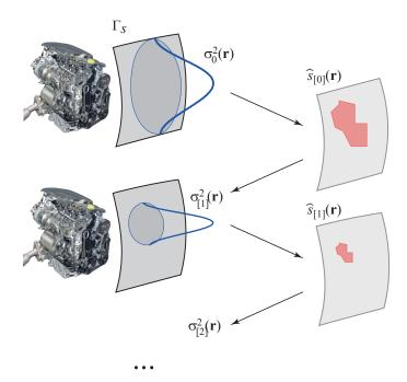
Figure 5: Principle of Iterated Bayesian Focusing: the reconstructed source  $\hat{s}_{[k]}(\mathbf{r})$  at the current iteration k is used to refine the aperture function  $\sigma_{[k+1]}^2(\mathbf{r})$  used in the next iteration.
