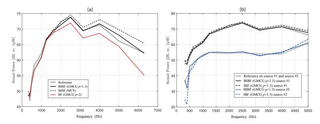
Figure 20: a) Overall sound power spectra estimated with Iterated Bayesian Focusing, with the MCS (a = b = 0.01) and GMCG (p = 1.3) priors, compared to Bayesian Focusing and to the intensity probe reference. b) Sound power spectra of each source estimated with Iterated Bayesian Focusing and Broadband Iterated Bayesian Focusing, with the GMCG (p = 1.3) prior.
