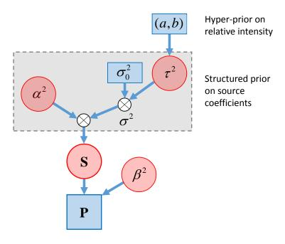
Figure 8: Directed graph of the hierarchical model for inferring **S**. Unknown parameters to infer are shown in circles and known quantities in rectangles. Note that **P** and **S** can be replaced by the CSM  $\mathbb{S}_{pp}$  and the source power spectrum  $S_{qq}$ .
