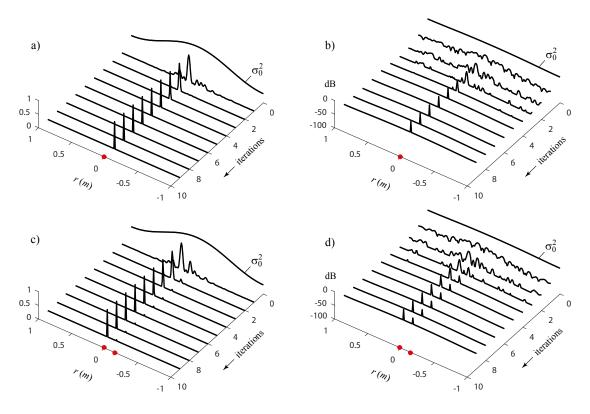
Figure 9: Update of the aperture function  $\sigma_{q,[k]}^2$  with respect to iteration numbers k=0,...,9 for the MCS prior. The zeroth iteration corresponds to the initial aperture function  $\sigma_{q,0}^2$ . Configurations with a-b) one monopole at r=0 m and c-d) two incoherent monopoles at r=0 m and r=-0.05 m (shown by red dots) with relative levels in the ratio 0.04. The two columns relate to linear and dB scales, respectively.
