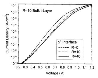
FIG. 1. Evolution of  $J_D-V$  characteristics for p-i-n cell structures with 0.4  $\mu$ m, R=10 a-Si:H i-layers when the p/i interface R value is increased from R=0 to 40.
