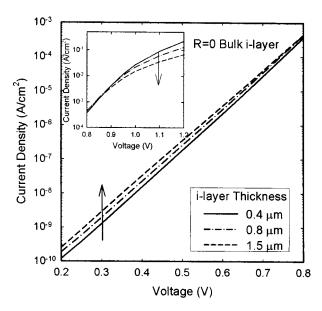
FIG. 2. The  $J_D-V$  characteristics of p-i-n cell structures with 0.4-, 0.8-, and 1.5- $\mu$ m-thick a-Si:H bulk i-layers and 200-Å-thick R=40 a-Si:H i-layers incorporated at the p/i interface. Shown in the inset is the opposite trend in the currents with thickness, when carrier transport is determined by drift rather than diffusion.
