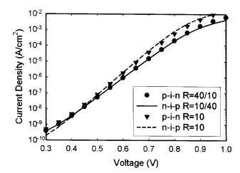
FIG. 3. The  $J_D-V$  characteristics of p-i-n and n-i-p cell structures with 0.4- $\mu$ m, R=10 i-layers, and with R=10 or R=40 a-Si:H at the p/i interfaces.
