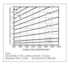
Figure 4: LCOE for energy output versus initial cost of the system for a zero interest loan, discount rate of 4.5%, degradation rate of 0.5%/yr and 30 year lifetime.
