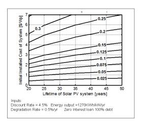
Figure 3: LCOE for lifetime of solar PV system versus initial cost of the system for a zero interest loan, discount rate of 4.5%, degradation rate of 0.5%/yr and energy output of 1270 kWh/kW.
