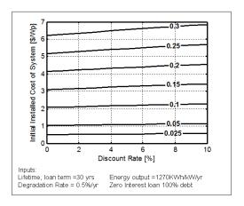
Figure 2: LCOE in  $\$ /kWh for solar PV system varying system costs and discount rates assuming zero interest loan, 30 year lifetime, degradation rate of 0.5%/yr and Energy output of 1270 kWh/kW/yr.
