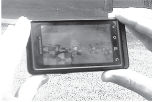
Fig. 4. Energy Wars Mobile prototype: visualisation of the virtual radiation markers using augmented reality markup.
