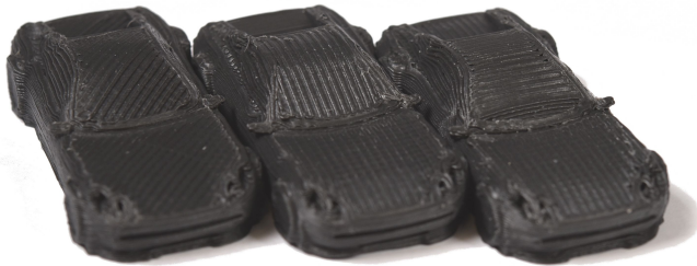
Fig. 15. Different toolpath orientations for the top layers in curved slicing result in different surface finish. The visible stripes are shallower than the layer thickness, yet they create a visual effect that is detrimental to perceived quality. The effect also depends on lighting and view angle.
