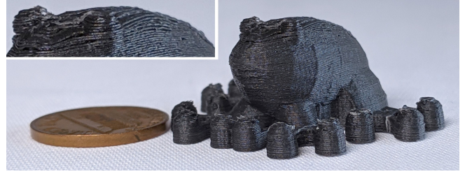
Fig. 8. Small frog model printed with curved slicing on an Anet A8 printer, with a 0.4mm nozzle and 103 layers between 0.3mm and 0.05mm. Layers at the top smoothly follow the curvature.
