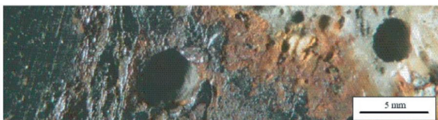
Figure 1: Microphotography and schematic representation of a transverse section of an iron rebar corroded in a hydraulic binder after Chitty (Chitty et al. 2006)
