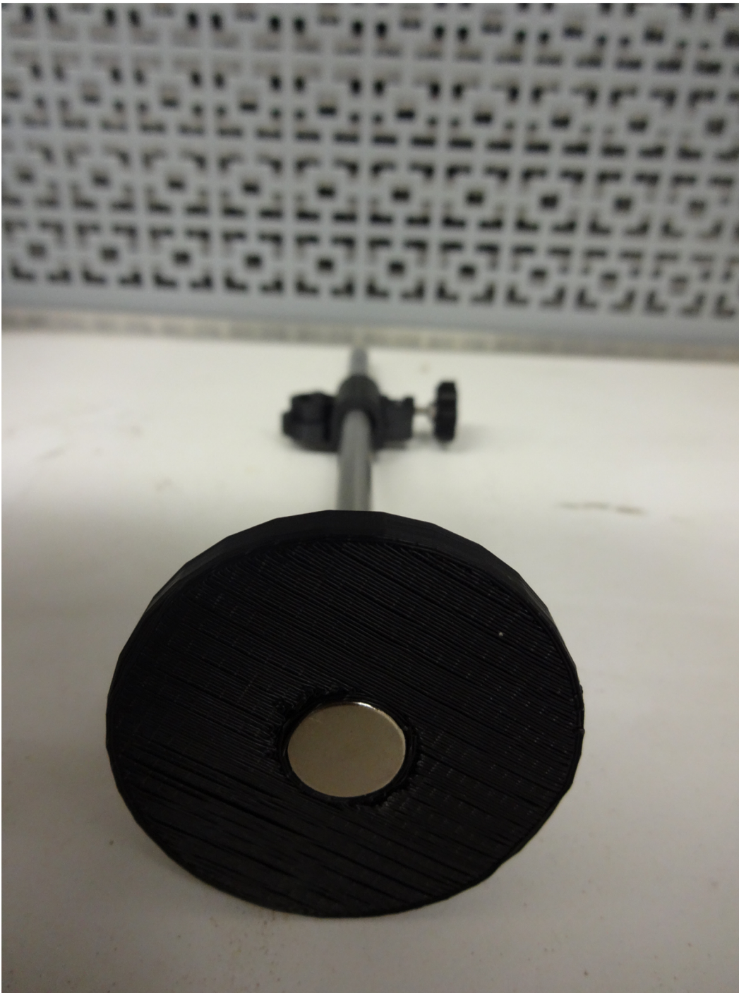
Figure 4. Magnetic optics base. doi:10.1371/journal.pone.0059840.g004
