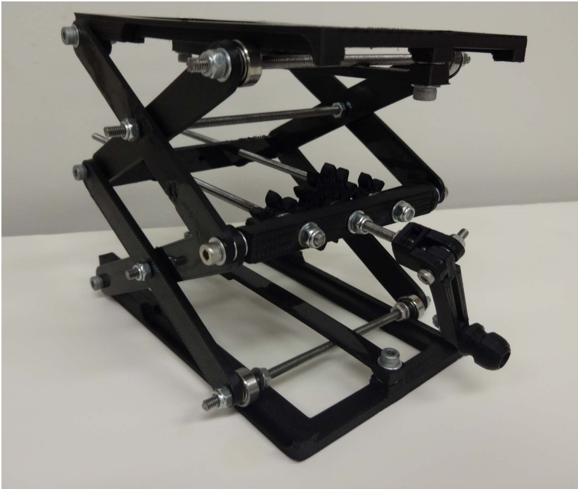
Figure 9. Open-source lab jack. doi:10.1371/journal.pone.0059840.g009
