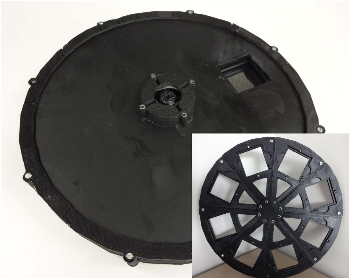
Figure 10. Parametric automated filter wheel changer. doi:10.1371/journal.pone.0059840.g010
