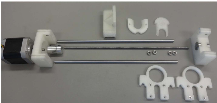
Figure 3. Exploded view of Open-Source Syringe Pump. doi:10.1371/journal.pone.0107216.g003
