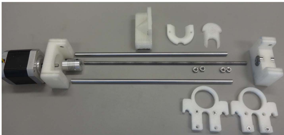
Figure 3. Exploded view of Open-Source Syringe Pump. doi:10.1371/journal.pone.0107216.g003
