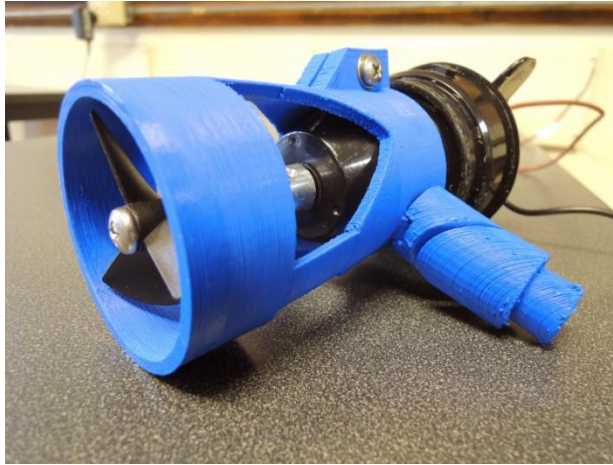
Figure 9. High School Student ROV Project Design
