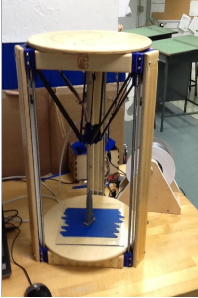
Figure 10. Customized MOST Delta RepRap
