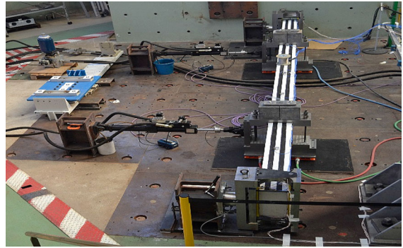
Figure 18 Quasi-static experimental setup on strong-floor
