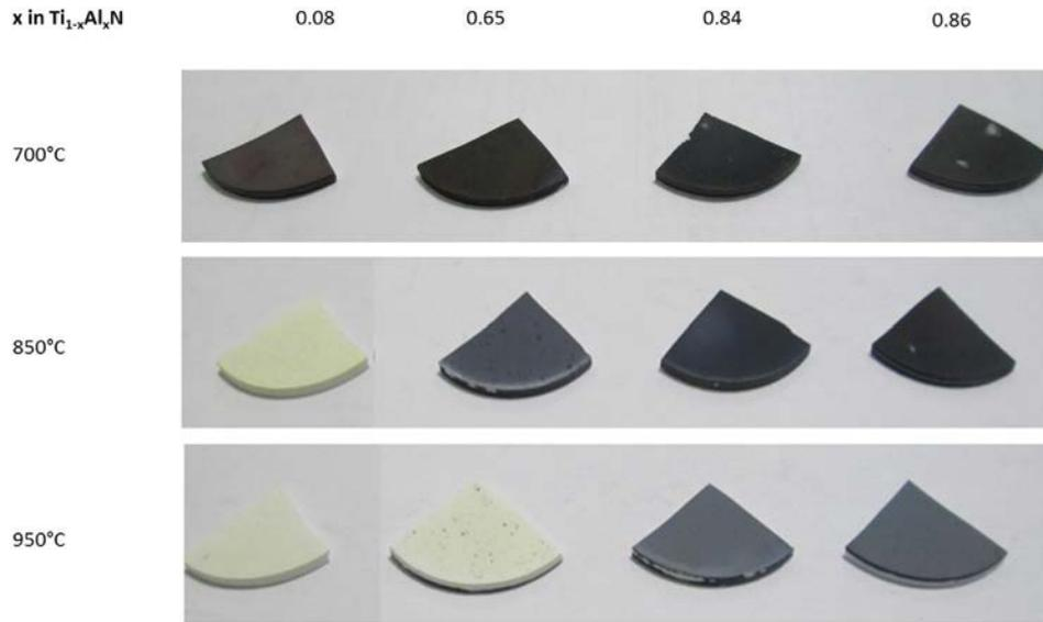
Fig. 9. Optical images of the Ti<sub>1-x</sub>Al<sub>x</sub>N coatings deposited on Al<sub>2</sub>O<sub>3</sub> substrates after oxidation during 1 h in air between 700 °C and 950 °C.
