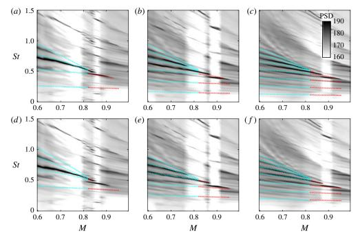
FIGURE 13. Refined tone-frequency predictions using vortex-sheet dispersion relations; assuming resonance between Kelvin–Helmholtz  $k^+$  and  $k^-$  jet modes, under out-of-phase reflection (a-c) and in-phase reflection (d-f) conditions; and assuming high-frequency cutoff due to trapped, non-reflecting  $k_{TH}^-$  jet modes in the range  $0.6 \le M \le 0.82$ , and due to cutoff of  $k_p^-$  jet modes in the range  $0.82 < M \le 1$ . From left to right: L/D=2, 3 and 4.
