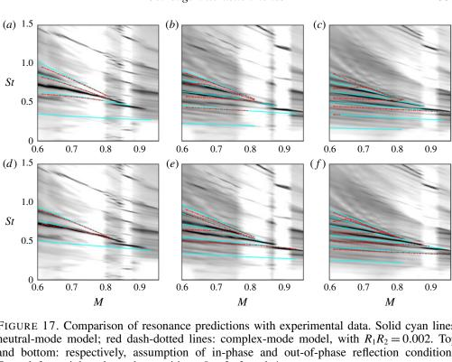
FIGURE 17. Comparison of resonance predictions with experimental data. Solid cyan lines: neutral-mode model; red dash-dotted lines: complex-mode model, with  $R_1R_2 = 0.002$ . Top and bottom: respectively, assumption of in-phase and out-of-phase reflection conditions. From left to right: plate-edge positions L = 2, 3 and 4.
