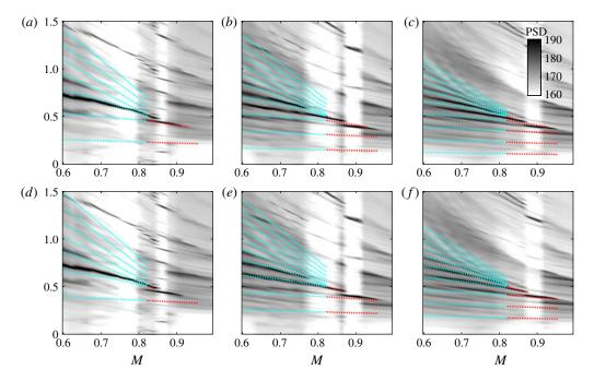
FIGURE 7. Tone-frequency predictions using vortex-sheet dispersion relations and assuming resonance between  $k_{KH}^+$  and  $k^-$  jet modes, with out-of-phase (a-c) and in-phase (d-f) reflection conditions. From (a-c) to (d-f) L/D=2, 3 and 4. Cyan: resonance between  $k_{KH}^+$  and  $k_{TH}^-$ ; red: resonance between  $k_{KH}^+$  and  $k_p^-$ .
