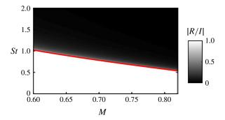
FIGURE 9. Reflection coefficient, |R/I|, for a  $k^-$ , soft-walled duct mode impinging on nozzle plane. The red line shows the cut-on frequency. At frequencies below this line, the incident wave is evanescent; above it is propagative, but has zero reflection coefficient: it is entirely transmitted into the nozzle as a rigid-walled duct  $k^-$  plane wave.
