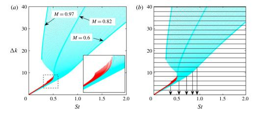
FIGURE 6. (a) Value of  $\Delta k$  between  $k_{KH}^+$  Kelvin–Helmholtz mode and all  $k^-$  jet modes in range  $0.6 \leqslant M \leqslant 0.97$ . (b) Illustration of resonance-frequency identification (showing frequency squeezing) for L/D=3, M=0.6 and out-of-phase reflection conditions: horizontal lines show values of  $\Delta k$  (4.8) for L/D=3.
