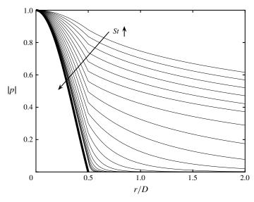
FIGURE 8. Thin lines: pressure eigenfunctions associated with  $k_{TH}^-$  jet modes at M = 0.6, in frequency range  $0.3 \le St \le 1.1$  (top-most line: St = 0.3; bottom-most line: St = 1.2). Thick line: soft-walled duct mode of radial order 1.
