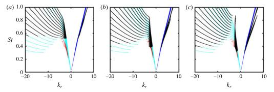
FIGURE 18. Eigenvalue branch deformation in Mach number range,  $0.61 \le M \le 0.93$ . Cyan, red and blue lines (neutral-mode model): respectively,  $k_{TH}^-$ ,  $k_p^-$  and  $k_{KH}^+$ . Black dots: complex-mode model for  $R_1R_2 = 0.002$ .
