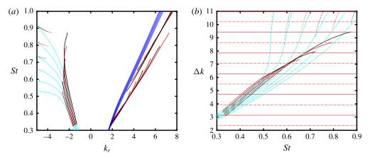
FIGURE 20. Zoom showing effect of the invalid saddle point discussed by Towne *et al.* (2017) (cf. figure 12(d) in that paper) on: resonance-eigenvalue branch deformation (a) and frequency prediction (b) using complex-mode model with  $R_1R_2 = 0.002$  and L = 4. From left to right: L = 2, 3 and 4.
