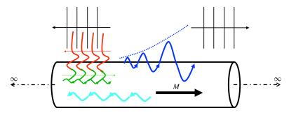
FIGURE 4. Schematic depiction of waves supported by cylindrical vortex sheet; colours correspond to those of figure 5.
