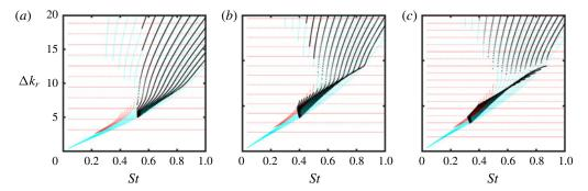
FIGURE 19. Resonance-frequency prediction with complex-mode model for  $R_1R_2 = 0.002$ ; resonance frequencies are given by intersection of horizontal red lines (solid and dash-dotted: respectively, in-phase and out-of-phase reflection conditions) and black-dotted lines. From (a) to (c) L = 2, 3 and 4.
