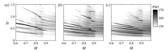
FIGURE 3. Power-spectral-density maps estimated from acoustic pressure recordings on the shielded side of the plate, by microphone m2 (cf. figure 1), and for the same three streamwise edge positions considered in figure 2.
