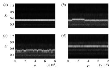
FIGURE 15. Time-frequency scalograms (grey scale shows wavelet-coefficient amplitudes) showing examples of four kinds of behaviour. (a) (M, L/D) = (0.8, 3): dominance of a single resonance cycle, despite the existence of two nearby possibilities; (b) (M, L/D) =(0.8, 4): slow competition between neighbour resonance cycles; (c) (M, L/D) = (0.78, 4): fast competition between neighbour resonance cycles; (d) (M, L/D) = (0.6, 2): co-existence of neighbour resonance cycles.
