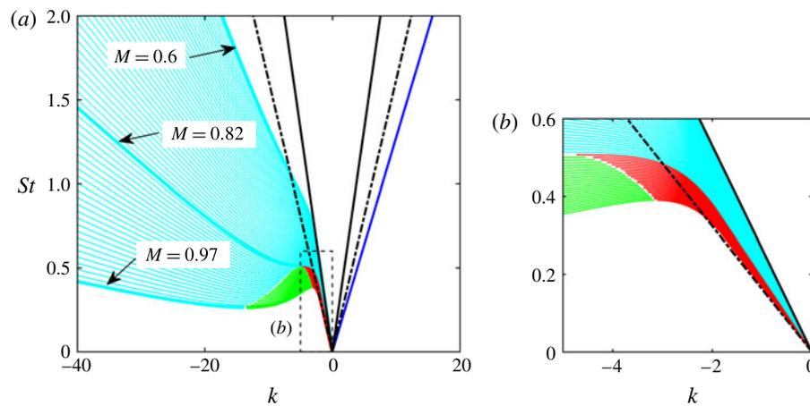
FIGURE 5. Vortex-sheet dispersion relations in the range  $0.6 \leq M \leq 0.97$ . Blue:  $k_{KH}^+$  Kelvin–Helmholtz modes; cyan in range  $0.6 \leq M \leq 0.82$ :  $k_{TH}^-$  modes (Tam & Hu 1989); cyan in range  $0.82 < M \leq 0.97$ :  $k_d^-$  modes (Towne *et al.* 2017); red and green, respectively:  $k_p^+$  and  $k_T^+$  acoustic jet modes (Towne *et al.* 2017); black:  $k^+$  and  $k^-$  free-stream sound waves (solid:  $M = 0.6$ ; dash-dot:  $M = 0.97$ ).
