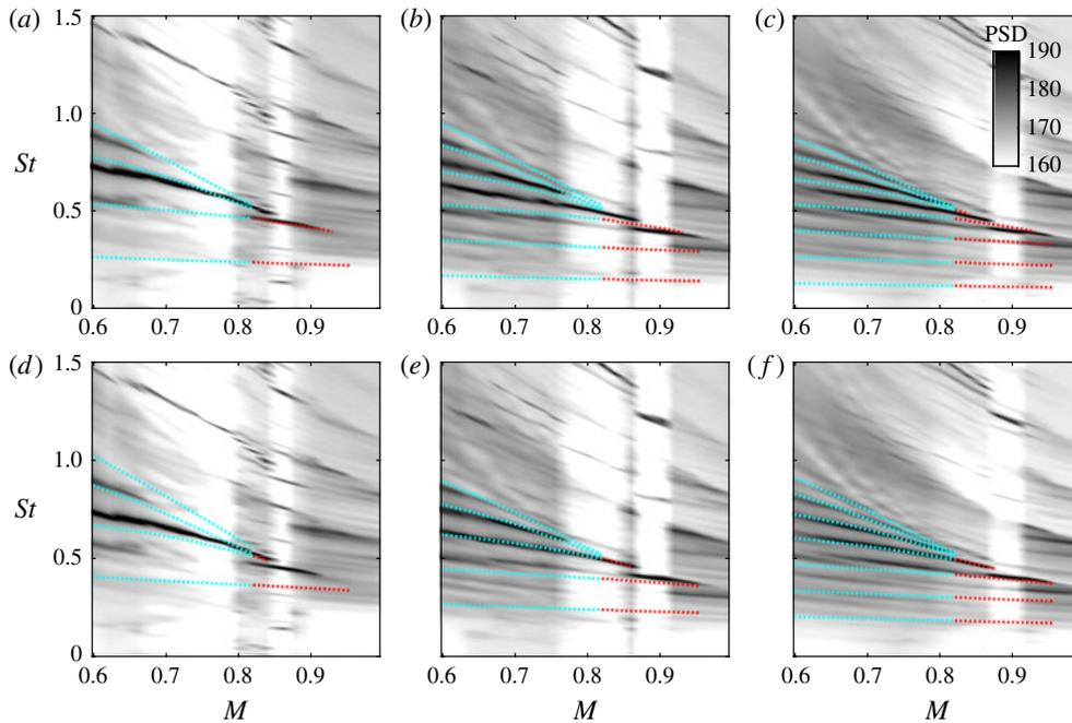
FIGURE 13. Refined tone-frequency predictions using vortex-sheet dispersion relations; assuming resonance between Kelvin–Helmholtz  $k^+$  and  $k^-$  jet modes, under out-of-phase reflection (a–c) and in-phase reflection (d–f) conditions; and assuming high-frequency cutoff due to trapped, non-reflecting  $k_{TH}^-$  jet modes in the range  $0.6 \leq M \leq 0.82$ , and due to cutoff of  $k_p^-$  jet modes in the range  $0.82 < M \leq 1$ . From left to right:  $L/D = 2, 3$  and  $4$ .
