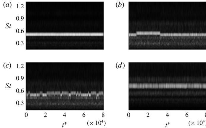
FIGURE 15. Time–frequency scalograms (grey scale shows wavelet-coefficient amplitudes) showing examples of four kinds of behaviour. (a)  $(M, L/D) = (0.8, 3)$ : dominance of a single resonance cycle, despite the existence of two nearby possibilities; (b)  $(M, L/D) = (0.8, 4)$ : slow competition between neighbour resonance cycles; (c)  $(M, L/D) = (0.78, 4)$ : fast competition between neighbour resonance cycles; (d)  $(M, L/D) = (0.6, 2)$ : co-existence of neighbour resonance cycles.
