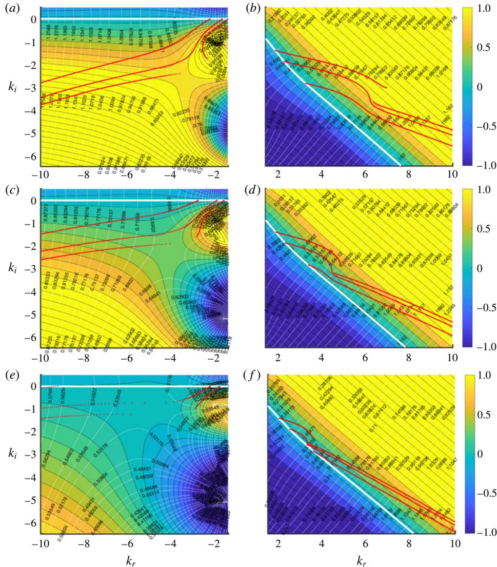
FIGURE 21. Vortex-sheet solutions,  $\omega(k)$ . The colour map shows  $\omega_i$ ; white isocontours show  $St = \omega_r/2\pi$ . Red dots indicate  $k^-$  (left plot) and  $k^+$  (right plot) modes satisfying the resonance amplitude constraint (B 8). From top to bottom:  $M = 0.6, 0.7$  and  $0.8$ . Solid white lines show neutral-mode model branches ( $\omega_i = 0$ ).
