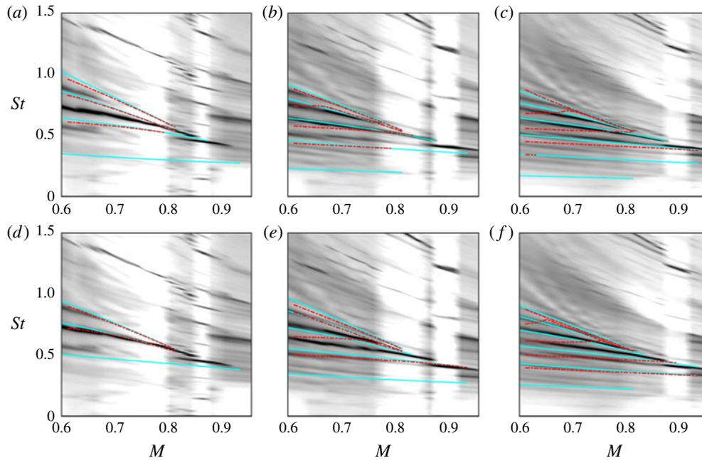
FIGURE 17. Comparison of resonance predictions with experimental data. Solid cyan lines: neutral-mode model; red dash-dotted lines: complex-mode model, with  $R_1 R_2 = 0.002$ . Top and bottom: respectively, assumption of in-phase and out-of-phase reflection conditions. From left to right: plate-edge positions  $L = 2, 3$  and  $4$ .
