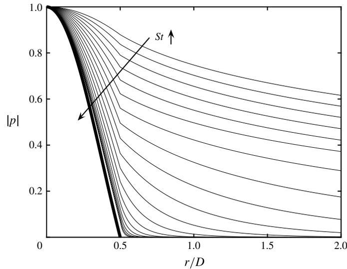
FIGURE 8. Thin lines: pressure eigenfunctions associated with  $k_{TH}^-$  jet modes at  $M = 0.6$ , in frequency range  $0.3 \leq St \leq 1.1$  (top-most line:  $St = 0.3$ ; bottom-most line:  $St = 1.2$ ). Thick line: soft-walled duct mode of radial order 1.
