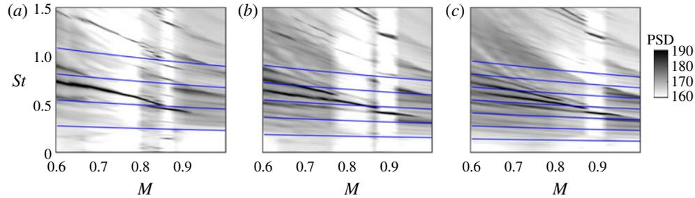
FIGURE 2. Power-spectral-density maps estimated from hydrodynamic, near-field pressure recordings (microphone  $m1$  in figure 1) for three streamwise edge positions, (a), (b) and (c): respectively,  $L/D = 2, 3$  and  $4$ . Blue lines show the poor resonance predictions based on coupling between downstream-travelling Kelvin-Helmholtz waves and upstream-travelling free-stream sound waves.
