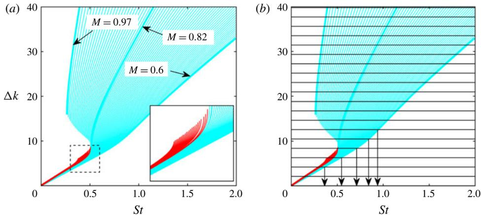
FIGURE 6. (a) Value of  $\Delta k$  between  $k_{KH}^+$  Kelvin–Helmholtz mode and all  $k^-$  jet modes in range  $0.6 \leq M \leq 0.97$ . (b) Illustration of resonance-frequency identification (showing frequency squeezing) for  $L/D = 3$ ,  $M = 0.6$  and out-of-phase reflection conditions: horizontal lines show values of  $\Delta k$  (4.8) for  $L/D = 3$ .
