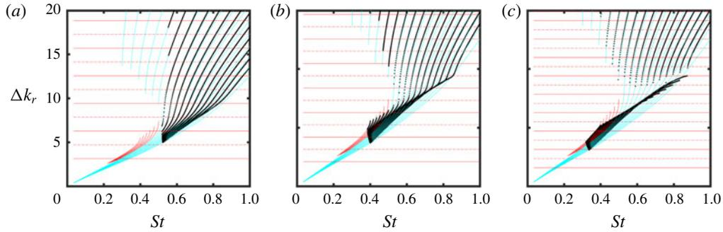
FIGURE 19. Resonance-frequency prediction with complex-mode model for  $R_1R_2 = 0.002$ ; resonance frequencies are given by intersection of horizontal red lines (solid and dash-dotted: respectively, in-phase and out-of-phase reflection conditions) and black-dotted lines. From (a) to (c)  $L = 2, 3$  and  $4$ .
