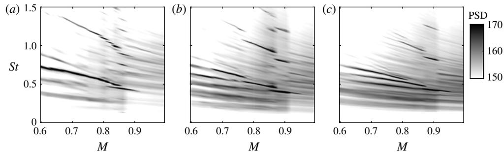
FIGURE 3. Power-spectral-density maps estimated from acoustic pressure recordings on the shielded side of the plate, by microphone  $m2$  (cf. figure 1), and for the same three streamwise edge positions considered in figure 2.
